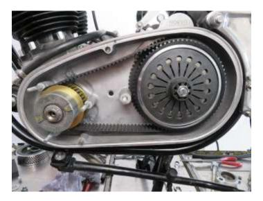
Install your alternator stator. Check the gap between the alternator stator and alternator rotor all the way around. The gap should be a minimum of 8 thou and a maximum of 20 thou.
