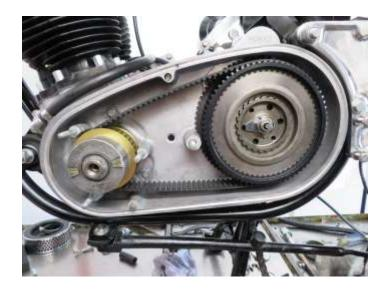
Install your clutch pressure plate and circlip using your clutch compressor tool.
