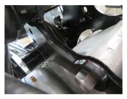
Tighten middle engine/cradle bolt to 30ft/lb. Tighten bottom engine/cradle bolt to 20ft/lb.
