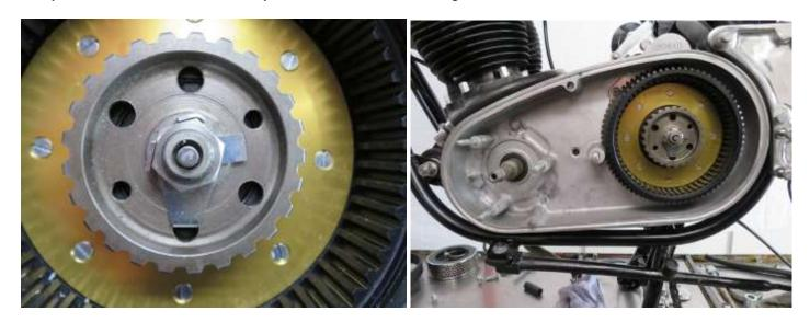
Slide on the front pulley that has been supplied.
