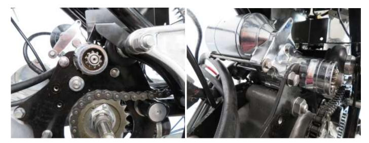
Install the bearing into the outrigger plate. Insert the outrigger plate onto the gearbox mainshaft.
