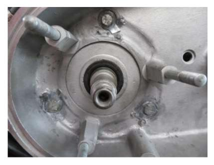
Tighten up the inner chaincase spacer to the engine plate. Install your tab washers to the clutch centre. Gently bend the tabs over and use your clutch centre tool to tighten the clutch centre bolt.
